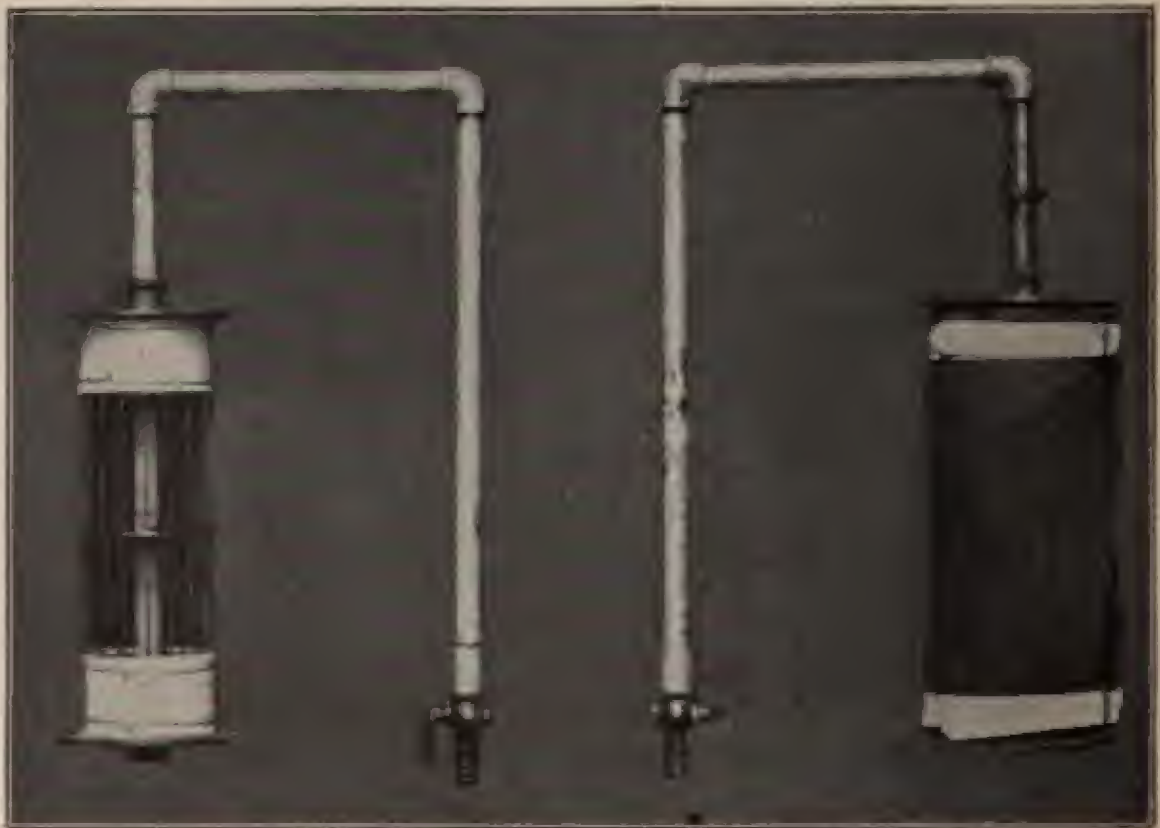
FIG. 60.—Filtering cylinder of the Darnall filter, with and without filtering cloth.
